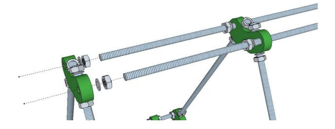
Slide the rods through the opposite side vertex. Thread the nuts up to the vertices on each side.
