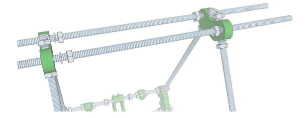
To each of the four ends of the threaded rod, add a washer, a nut and another washer.
